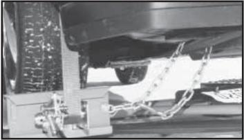
**Step 12.** Hook the towed vehicle safety chains to frame of vehicle directly above the area where the chains are mounted on the Kar Kaddy. Leave some slack in the chains to allow suspension movement of the towed vehicle.
